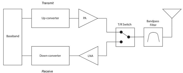
FIGURE 2. Alternative Simplified TDD Architecture
