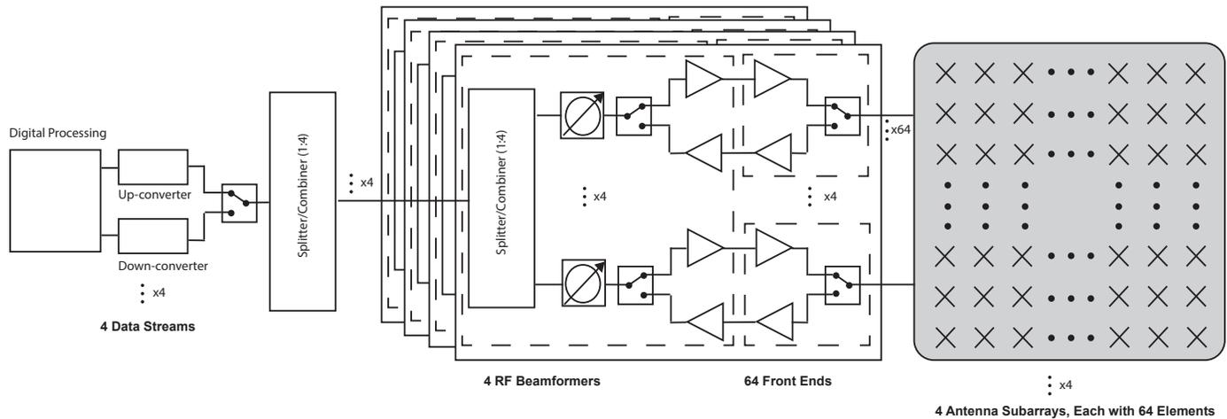
FIGURE 3. Simplified Hybrid Beamforming Architecture
