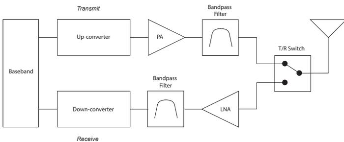
FIGURE 1. Simplified TDD Architecture
